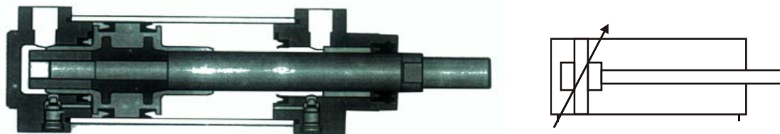
FIG.10 DOUBLE ACTING CYLINDER WITH END POSITION CUSHIONING
