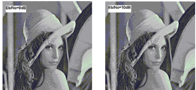
Fig. 6. Reconstructed images for AWGN Channel using QAM modulation with M=2 for E_b/N_0 = 9\text{dB} and 10\text{dB} .
