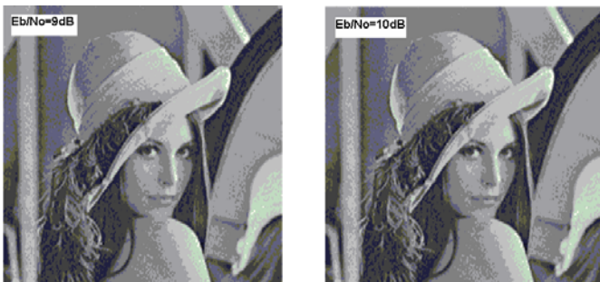
Fig. 5. Reconstructed images for AWGN Channel using PSK modulation with M=2 for E_b/N_0 = 9\text{dB} and 10\text{dB} .
