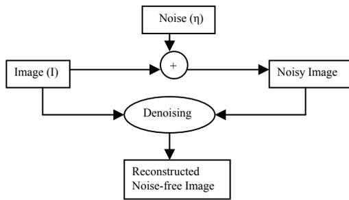
Fig. 1. Block diagram of Image Denoising Process
