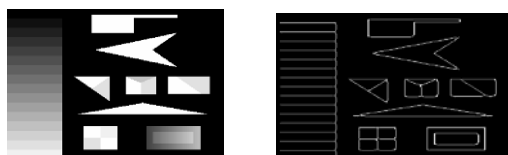
Figure 7: An image designed to test corner and edge detectors Figure 8: Output of the SUSAN edge finder ( t=10 ) given the test image.
