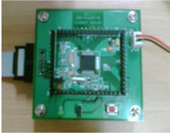
Fig.7. MSP 430F1612 Target Board
