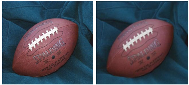
Fig. 7. Results from HDL simulation of averaging filter.
