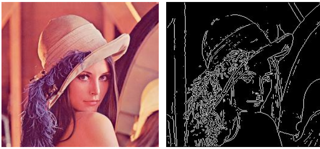
Fig. 10. Results from MATLAB simulation of Sobel edge detection technique
